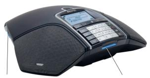
The **Konftel 300M** is a batteryoperated wireless conference phone that can be connected to mobile networks (GSM/3G) or PCs (USB).
