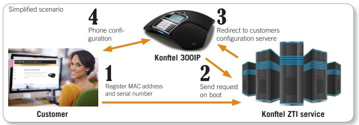
Zero Touch Installation is an add-in for auto-provisioning that is supported in the Konftel 300IP. It's basically about remote configuration of IP conference phones via a data file with settings. The devices download the file from a provisioning server, sometimes referred to as a device management server. The function is also used when centrally upgrading phone software.
